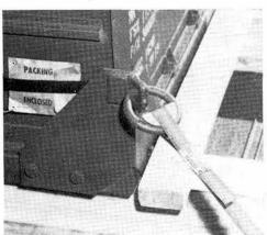
LINK AND SHACKLE INSERT, shown here fitting inside a ring on a special Sandia container, enables the use of commercial steel strapping to tie down Sandia shipments in rail cars and truck vans.
